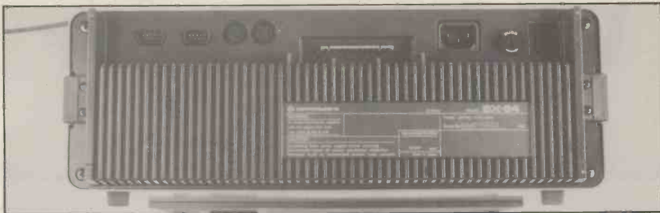
Two A/D interfaces, a printer connector and the DIN audio/video connectors are on the back, along with the power On/Off switch.
