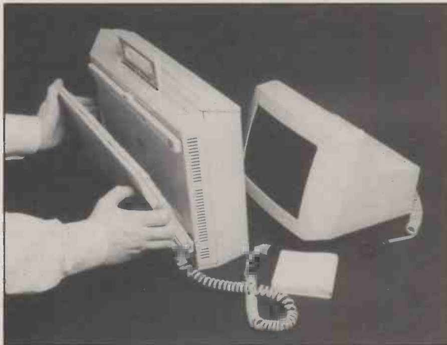
The keyboard clips under the main unit — but the display must be carried separately.
